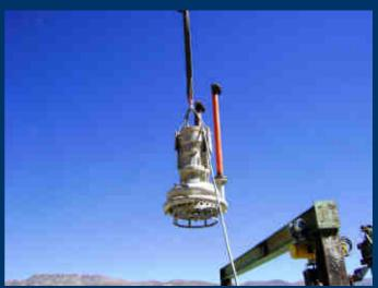
Pond Cleaning – Dragflow El35 With High Pressure Water Jet Ring
